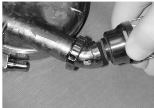
Figure 18 Attaching the New Inflow Valve Conduit to the inflow side of the LVAD by grasping the outlet bell graft nut and screwing it onto the Inlet Elbow.
