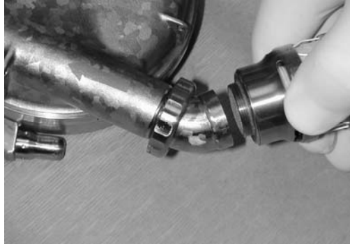
Figure 19 Attaching the New Inflow Valve Conduit to the inflow side of the LVAD by grasping the outlet bell graft nut and screwing it onto the Inlet Elbow.
