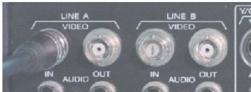
BNC connection to Line A VIDEO IN
